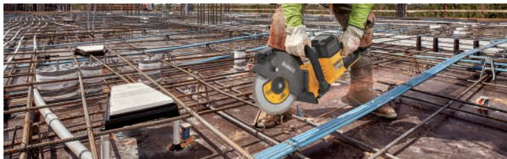
Makes fast and efficient single pass cuts and scores in concrete, pavestones, steel, and rebar.
